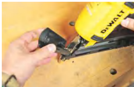
Each gun has a front access area for dealing with nail jams
